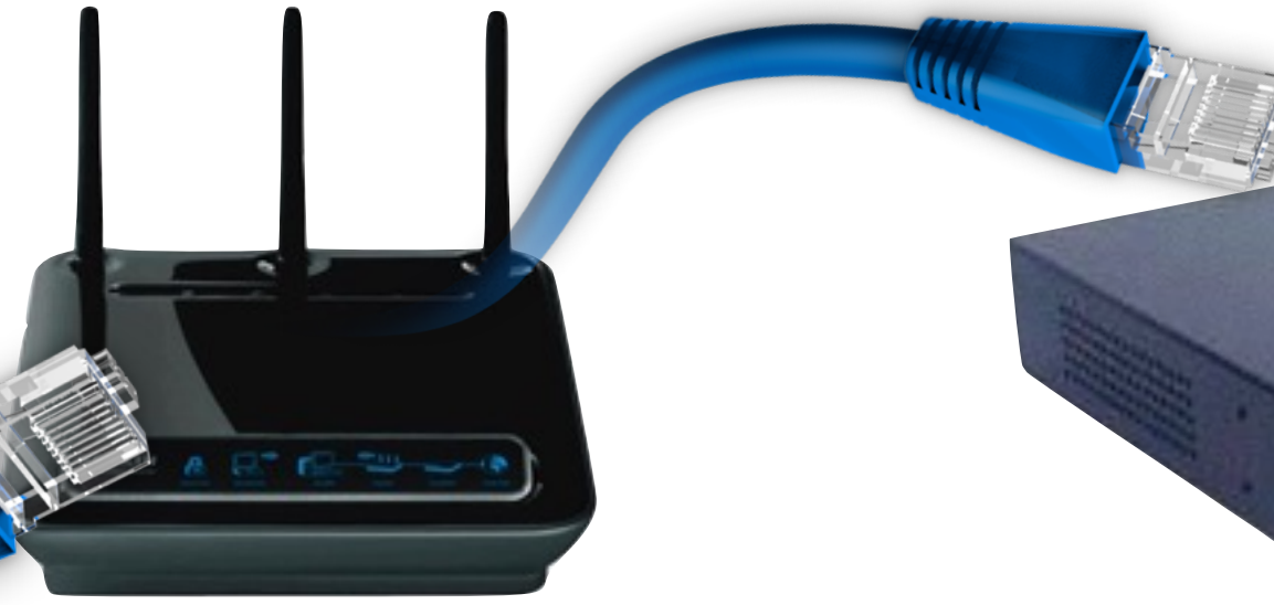
Wireless Router (Firewall)
